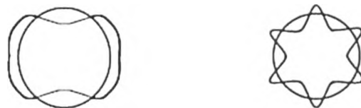
Figure 2-45. Circumferential buckling waves for n = 2 (left) and n = 6 (right)
