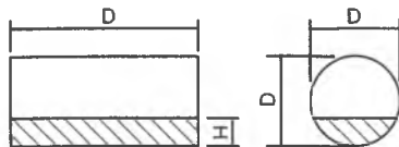
Coefficients for Partial Volumes of Horizontal Cylinders, C
